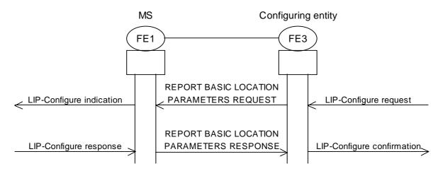
Figure 5.5: Basic configuration parameters reporting
